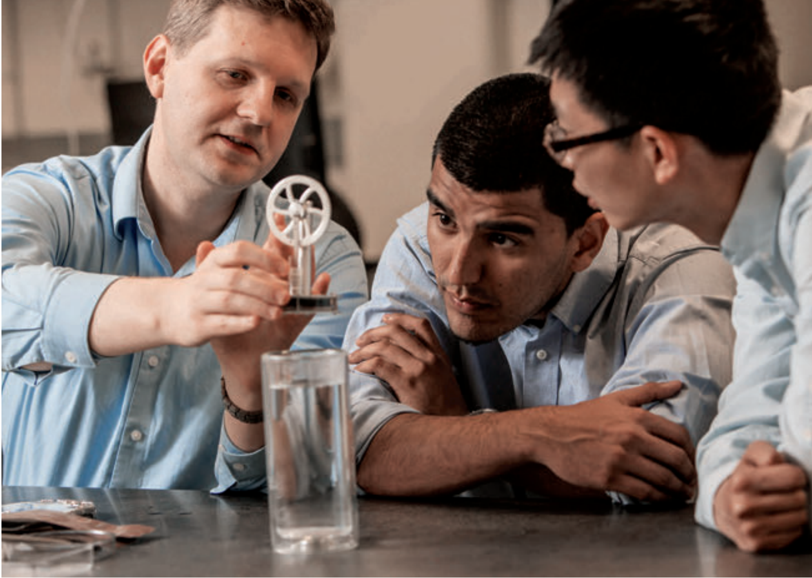
Bargatin demonstrates a Stirling engine with Chen Lin (right) and John Cortes (center), third- and second-year doctoral students, respectively. A Stirling engine can convert the energy from hot water (seen in the cup below the engine) into mechanical work, driving the crankshaft of the engine.
